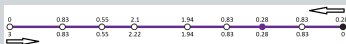
FIG.: Average arrival rates \lambda_j for every platform j , in passenger by second. The mean of those rates is 1.
